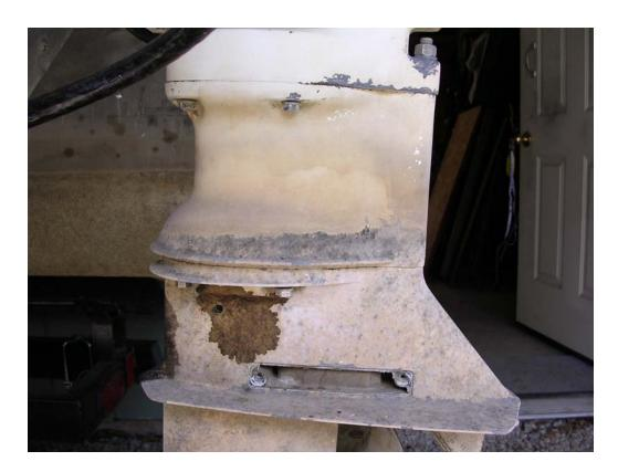
3. Now that you have the bolts loose you need to disconnect the shifting rod. On some outboards you disconnect the shifting rod underneath the block...on this motor which is a 28HP Johnson you have an access door. Note: This style is a pain in the butt in my humble opinion....see below.
