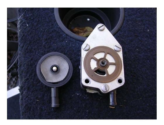
4. Fourth you'll have to remove the gasket and install a new one... FYI this fuel pump new was \$50. with shipping. The gasket is under \$10.
